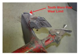
The outside tooth of this 4400-8E3 Earth Auger is severely worn from extended use. There is insufficient material remaining to secure a replacement outside tooth. The auger will now "bind" itself in the hole while digging and is no longer capable of digging an 8 inch diameter hole. The auger was removed from service and scrapped.
