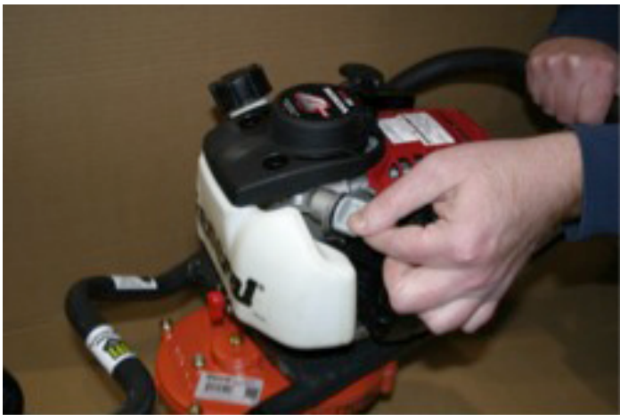
FIGURE 2 depicting the improper method to check oil level for the Honda GX35 engine.
