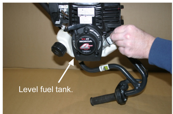
FIGURE 1. Note that fuel tank is positioned level or parallel relative with the surface.
