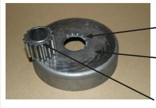
Markings indicate the high temperature brazing process properly bonded the clutch drum and pinion gear.
