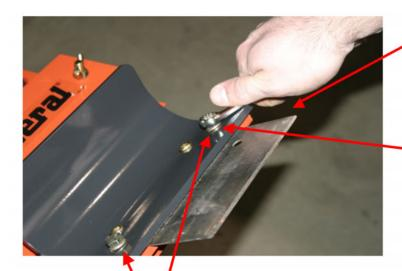
Note how close the hand is to the sharp blade edge. A slipping wrench can result in personal injury.
